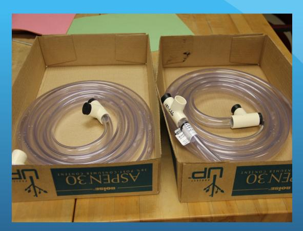
This is a picture of the set-up of the coiled tubes, which represents the loop within the geothermal system for the model.
